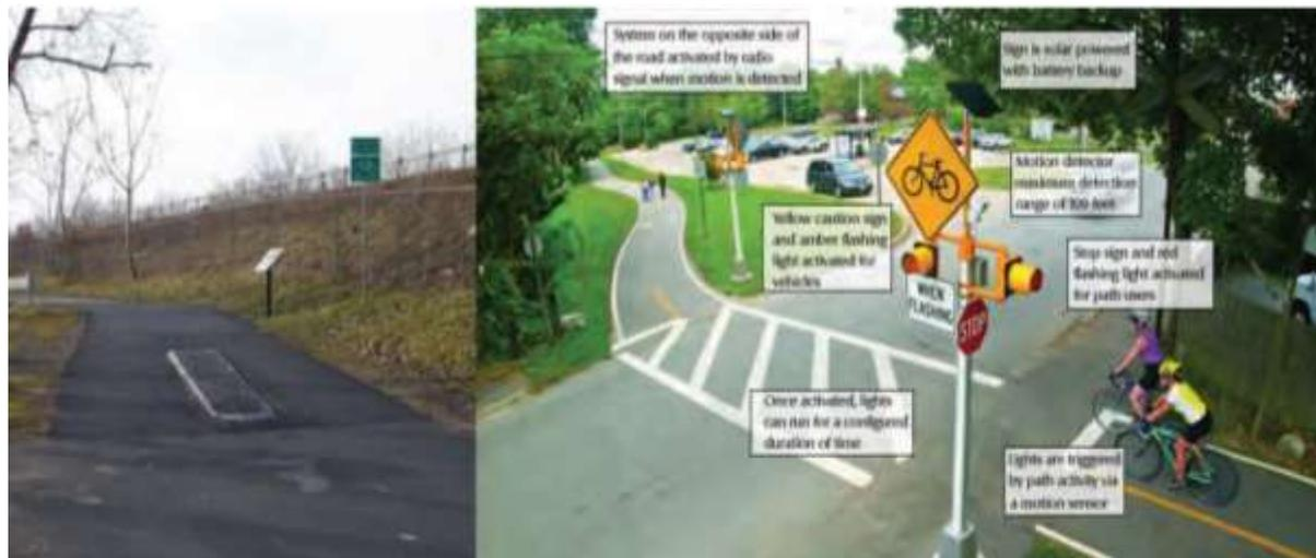
Figure 21: Trail crossing. Image Source: City of La Crosse Bicycle and Pedestrian Master Plan, 2012.
