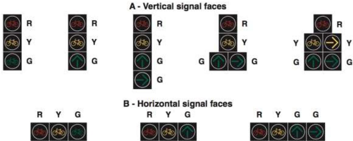
Figure 28: Signal Arrangements for Bicycle Lanes or mixed traffic. Image Source: FHWA Design Guide
