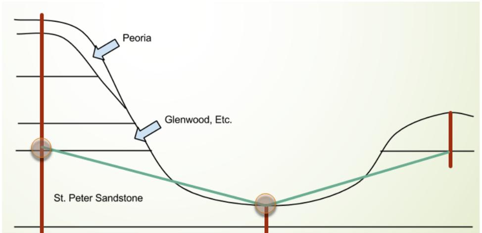
Figure 10 - The well drilling in the middle of the valley shown above has been exposed to erosion and causes noise in the upper elevation data interpolation. Such noise lowers local spatial autocorrelation and can degrade results.
